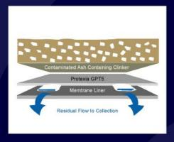
Migration of layers, which would reduce the load-bearing capacity of the system, is thereby avoided and at the same time water flow is maintained, consequently improving the stability and life of the entire construction.
